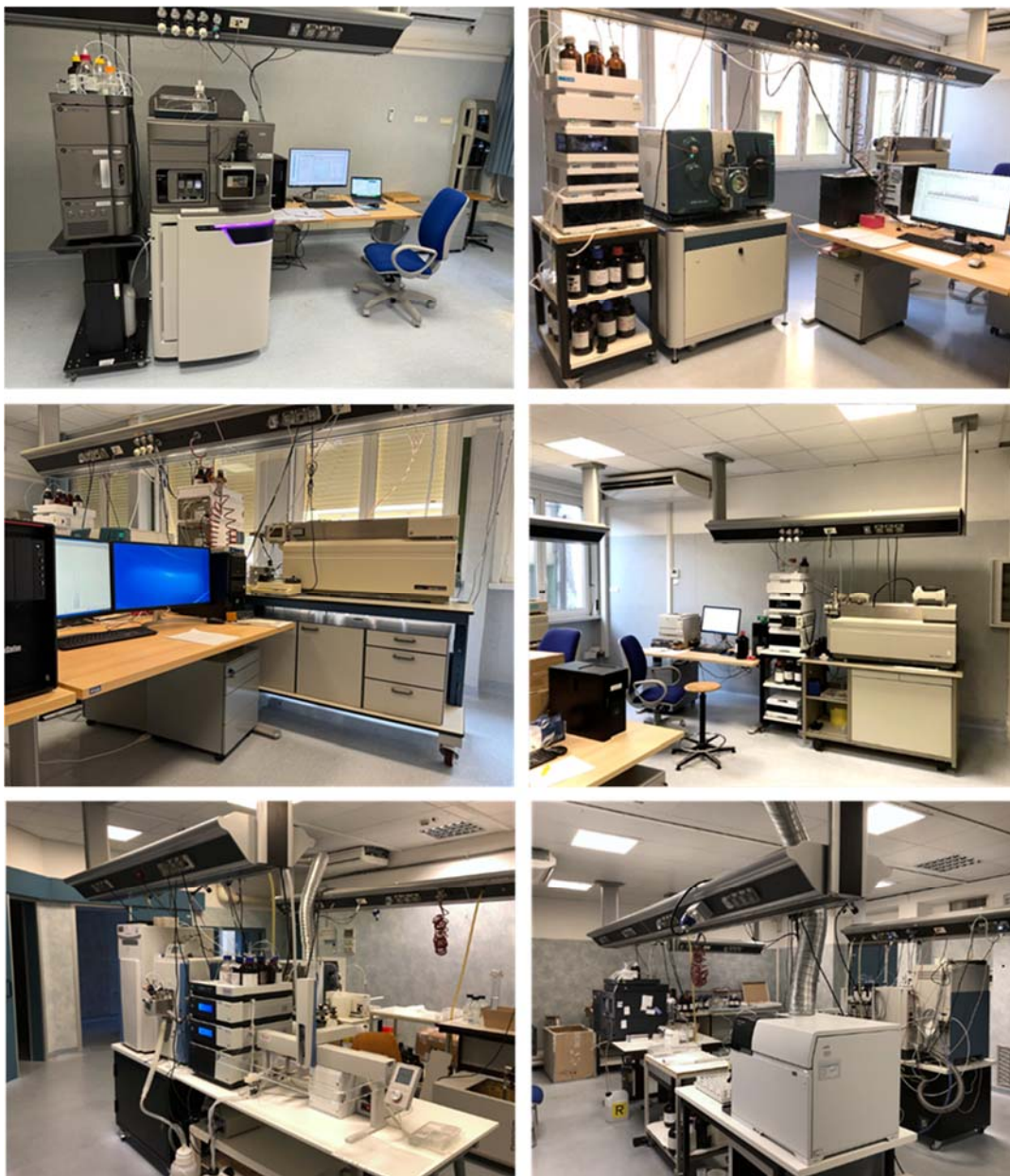
Figure 1. MS systems in the UniPi-AOUP LSM lab: Waters Synapt XS HR LC-Q-IMS-TOF mass spectrometer (upper-left) and Sciex QTrap 6500+ LC-Hybrid Tandem Quadrupole (upper-right), Sciex API 3000 LC-triple quadrupole mass spectrometer (middle-left), Sciex API 4000 LC-triple quadrupole mass spectrometer (middle-right), Thermo Scientific Q Exactive LC-Hybrid Quadrupole-Orbitrap-MS (lower-left), and Agilent 7900 ICP-MS (lower-right).
